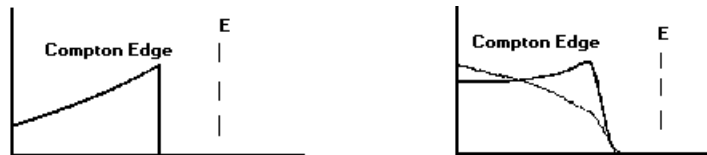
Figure 3. Theoretical and actual spectra produced by a plastic scintillator from a single 1 - MeV \gamma ray.
